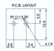
Current: 10A @ 300V Wire Range: Pin dimension CR: IR: Operating Ten Stripping Len: Torque: PCB holes:
